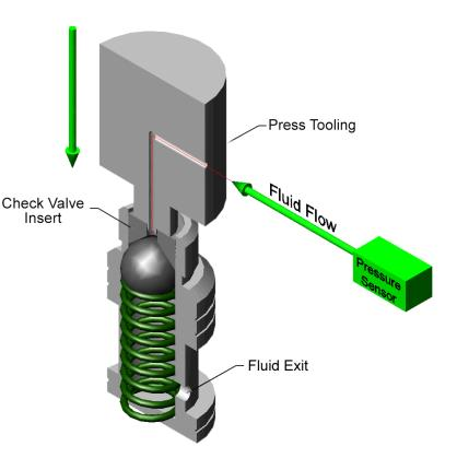
pressure by compressing the spring inside the valve to increase its resistance. The EMAP presses the valve seat into the valve body until the target release pressure of 1,000 psi is reached.
